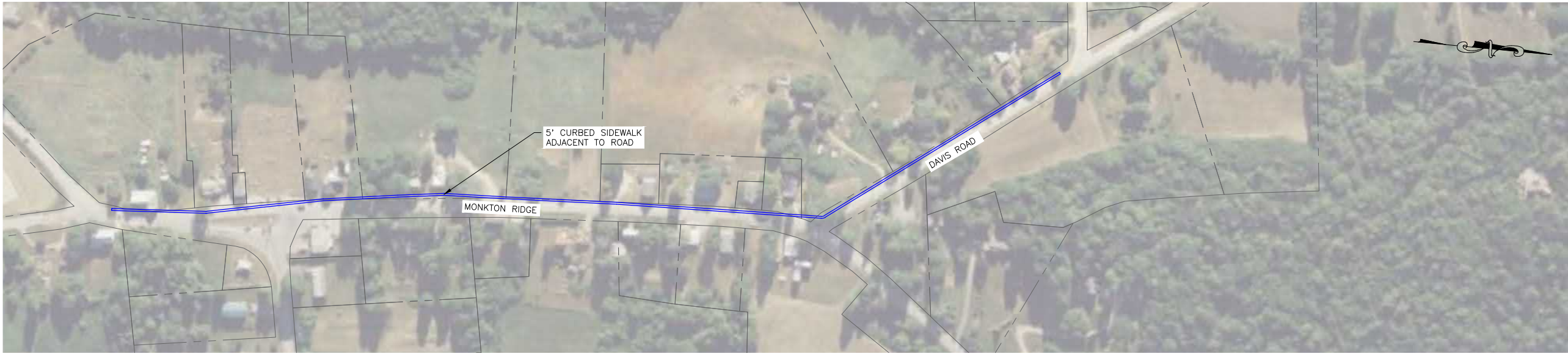
MONKTON RIDGE/ DAVIS ROAD ALTERNATIVE 1 5' CURBED CONCRETE SIDEWALK ADJACENT TO ROAD
