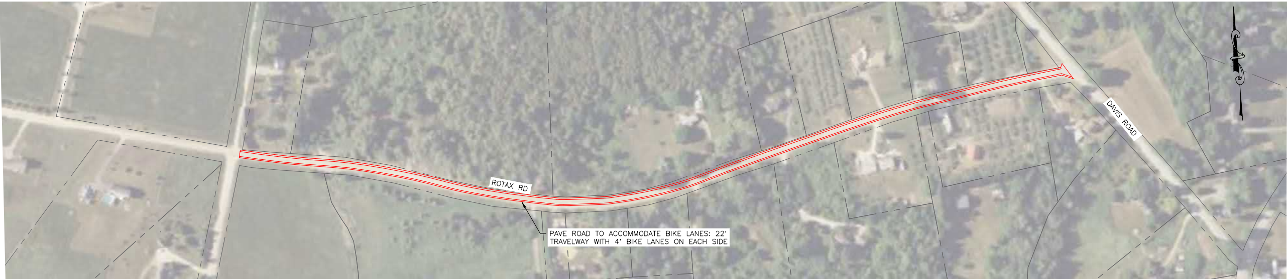
ROTAX ROAD ALTERNATIVE 2 PAVE ROAD AND PROVIDE 4' BIKE LANES ON BOTH SIDES OF ROAD
