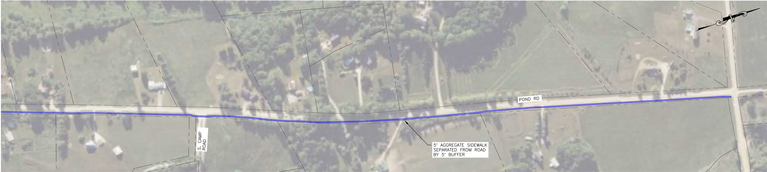
POND ROAD ALTERNATIVE 1 5' AGGREGATE SIDEWALK SEPARATED BY 5' BUFFER (NORTHERN SECTION)
