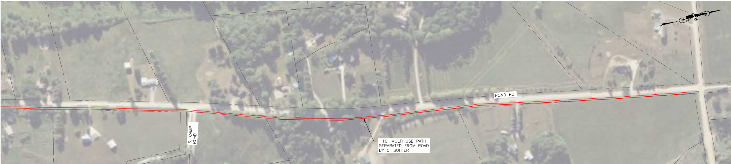
POND ROAD ALTERNATIVE 2 10' AGGREGATE MULTI-USE PATH SEPARATED BY 5' BUFFER (NORTHERN SECTION)
